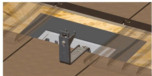
EcoFasten recommends following the TRI guidelines three-course sealing method. Start the three-course sealing method by applying a layer of roofing mastic over the edges of the tile hook sub-flashing.
